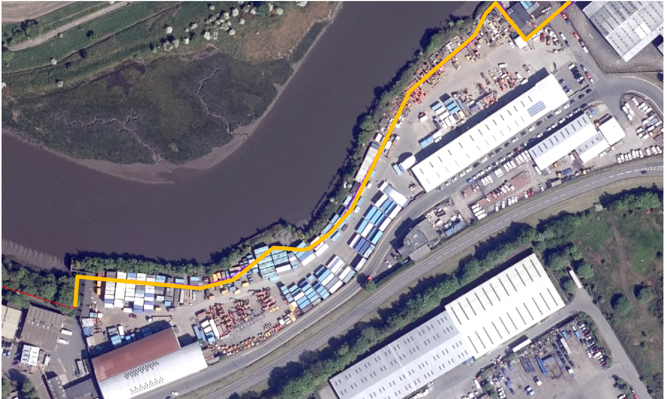
Figure 19 flood defence alignment through Jarvie Plant Yard
